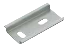
TS 35/7.5 mm according to EN 50022 (s = 1.0 mm)
